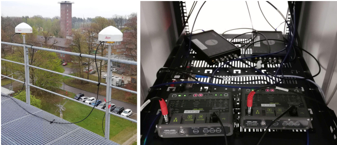
Fig. 2. GNSS antennas and receivers atop and inside Meitner building at PTB, respectively. From left to right: first antenna, second antenna, JAVAD OMEGA receivers in the front, Septentrio PolaRx5TR receivers in the back.
